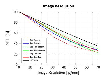
Modulation Transfer Function (MTF) vs. Image Resolution (wavelength range 486 nm - 656 nm), wf/N= 13, of cylindrical object of diameter 30 mm and height of 20 mm
